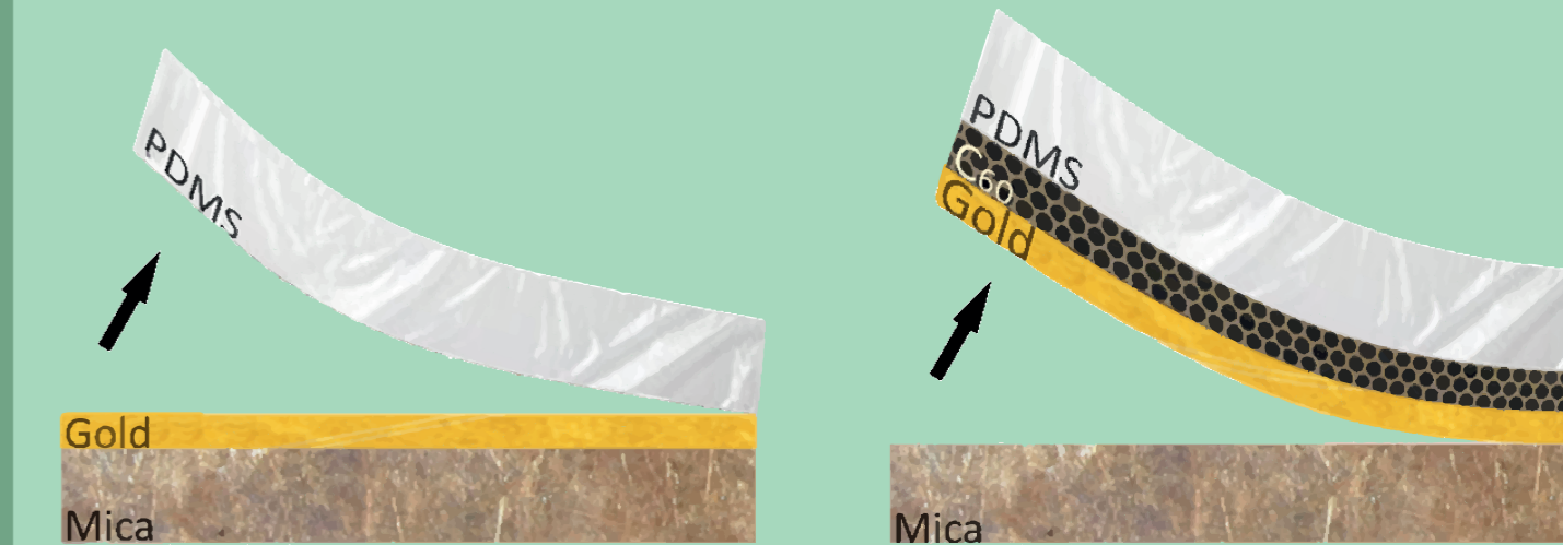
Figure 4: Peeling of PDMS off a gold / mica sample without and with a layer of C 60 . The adhesive properties of C 60 enable clean removal of the gold off the mica.
