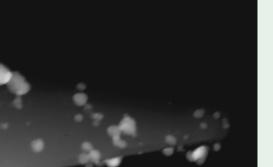
different incident laser powers. A coating of 3-amino-triethoxysilane (APTES) was used on some tips so that silver particles would preferentially bind to the surface.
