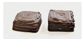
Sintered samples extruded at 50µl/min dried in air (left) and with a fan (right).
