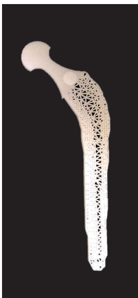
2D representation of a femoral stem component designed with an intelligently distributed material density.
