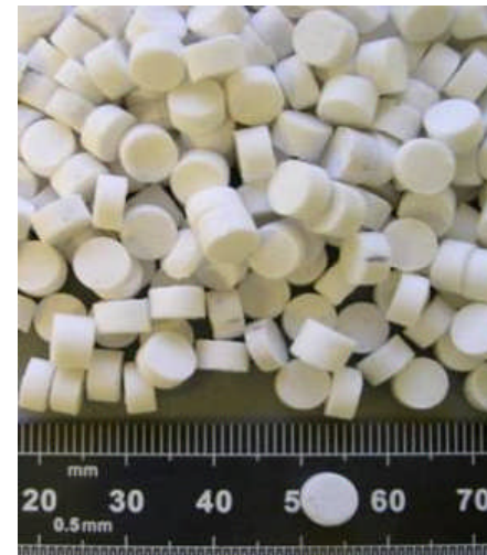
Pellets capturing CO 2 using amine polymer
