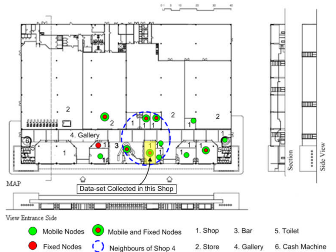
Figure 1: Map of the shopping mall with 13 shops, 18 mobile devices and 7 fixed devices involved in the experiment
