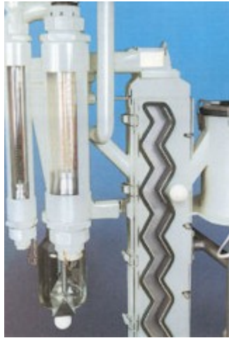
Figure 7: Zig-Zag Classifier (Source: www.hosokawamicron.com )
