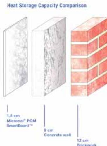
A Micronal® PCM SmartBoard™ only 1.5 cm thick features a thermal storage capacity identical to that of 9 cm concrete or 12 cm brickwork! Thus, it is the ideal building material for both refurbishment and modern lightweight construction.
