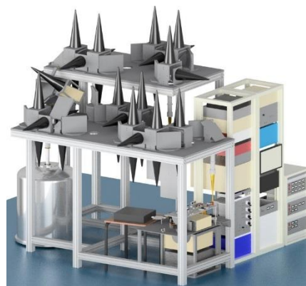
Figure 1: The HiPER spectrometer operates at 94 GHz, with a 1 GHz instantaneous bandwidth and an average B_1 \sim 40 MHz. It operates in induction mode, which gives the spectrometer low deadtime and high dynamic range. The black cones are high performance microwave loads, designed to largely eliminate system reflections.
