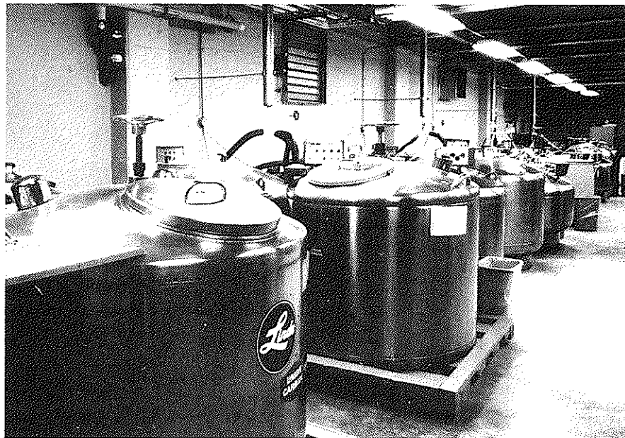
Figure 3. Liquid nitrogen (vapour phase) preservation containers at the American Type Culture Collection (ATCC).
