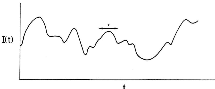
Fig. 1. Fluctuation in scattered intensity,  $I(t)$  with time,  $t$ . The variable  $\tau$  is defined as the "delay time." At short delay times, there is good correlation in the scattered intensity; at long delay times, poor correlation.
