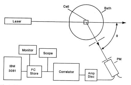
Fig. 3. Schematic dynamic light scattering apparatus (redrawn from ref. 16).  $\theta$ : scattering angle; Amp Disc: amplifier-discriminator; PM: photomultipliers; PC: IBM PC-compatible computer; IBM-3081: mainframe computer (only necessary for more sophisticated analyses).
