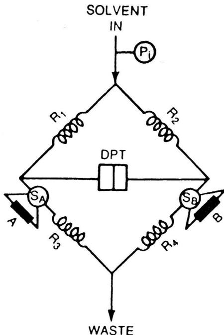
**Figure 1.3** Simplified schematic of pressure imbalance differential viscometer. Uses fluid analogue of a Wheatstone bridge electrical circuit to measure differential viscosity directly from the chromatography effluent.  $R_1$ – $R_4$  capillaries. A, B solvent reservoirs.  $P_i$ : inlet pressure. DPT: differential pressure transducer. From Haney *et al.* (1985a,b).
