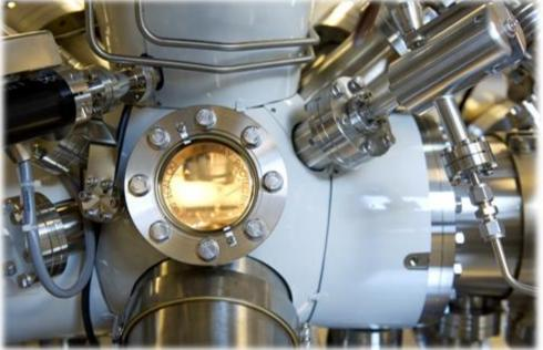
\* Analyse ionic liquids with the liquid phase photoelectron spectroscopy instrument (LiPPS) at the NNNC.
