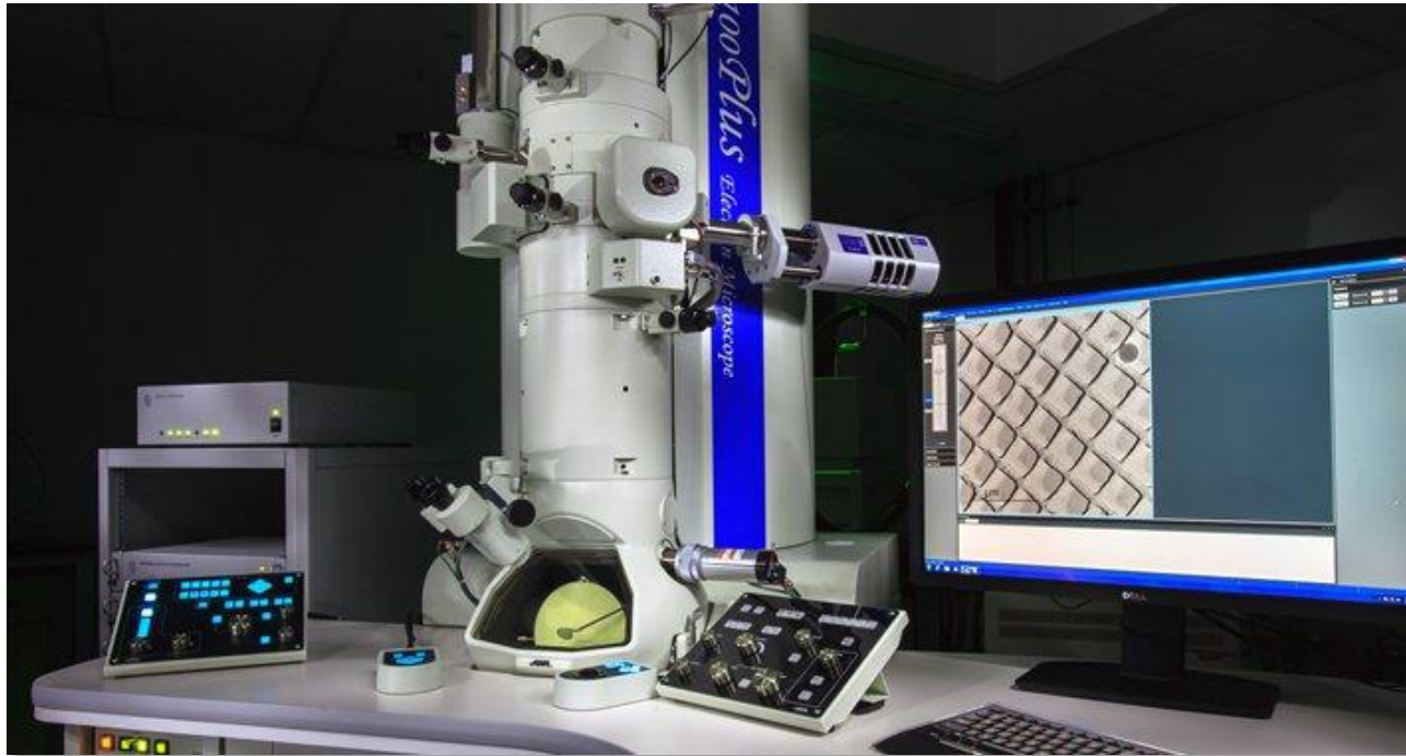
The versatile JEOL 2100+ TEM for nanostructural characterisation at the Nanoscale and Microscale Research Centre (nmRC), University of Nottingham
