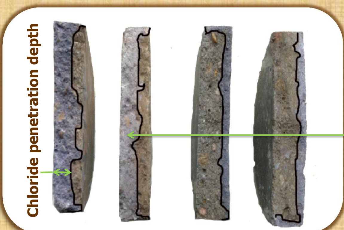
Chloride depth in different types of SCC in modified rapid chloride migration test
