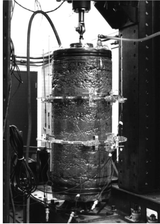
Constant Confining Pressure Apparatus (800 mm x 400 Ømm) for Testing Unbound Granular Materials
