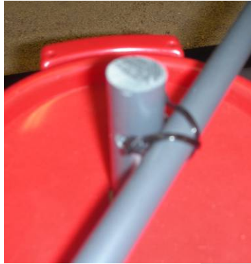
Figure 10.7: Stirring handle cable tied together.
