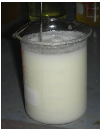
Figure 4.2: The effect of overly vigorous stirring.
