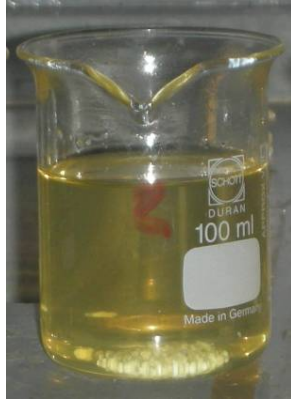
Figure 7.2: Meth-oxide solution with unreacted catalyst.
