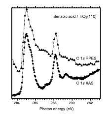
FIG. 6. Comparison of C 1s XAS and RPES for benzoic acid. In both cases the spectra have been corrected for a highly varied higher-order background (Ref. 14). The strong resonant photoemission signals at 285 eV and 288 eV photon energy indicate strong localization of the excited electron to the adsorbate. An assignment of the smaller peaks is not motivated, as the background (Ref. 14) easily induces smaller structures.
