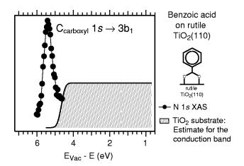
FIG. 5. Unoccupied density of states for benzoic acid for an XAS calibration which employs the ionization potential of the carboxylic C 1s. The only peak shown is that which is ascribed to a  $C_{carboxyl} \ 1s \rightarrow 3b_1$  excitation and which is found at approximately 1.7 eV ionization potential in Fig. 4(b).
