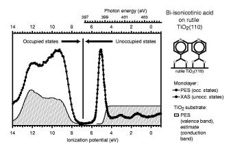
FIG. 1. Combination of valence photoemission spectra (PES), an x-ray absorption spectrum (XAS), and a substrate band gap estimate for a monolayer of bi-isonicotinic acid adsorbed on rutile  $TiO_2(110)$  to give an image of the electronic structure of the coreexcited adsorbate system. The spectra have been placed on a common energy scale; in addition, the photon energy scale of the x-ray absorption spectrum has been given.
