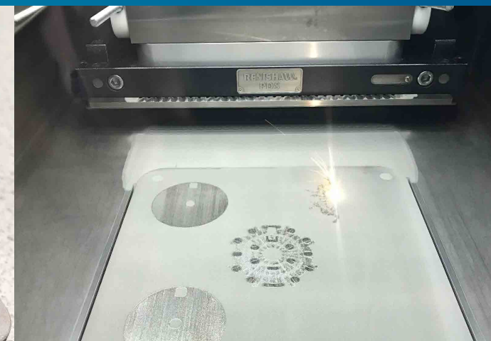
Additive manufacturing of Fe-Si soft magnetic components for an electric motor
