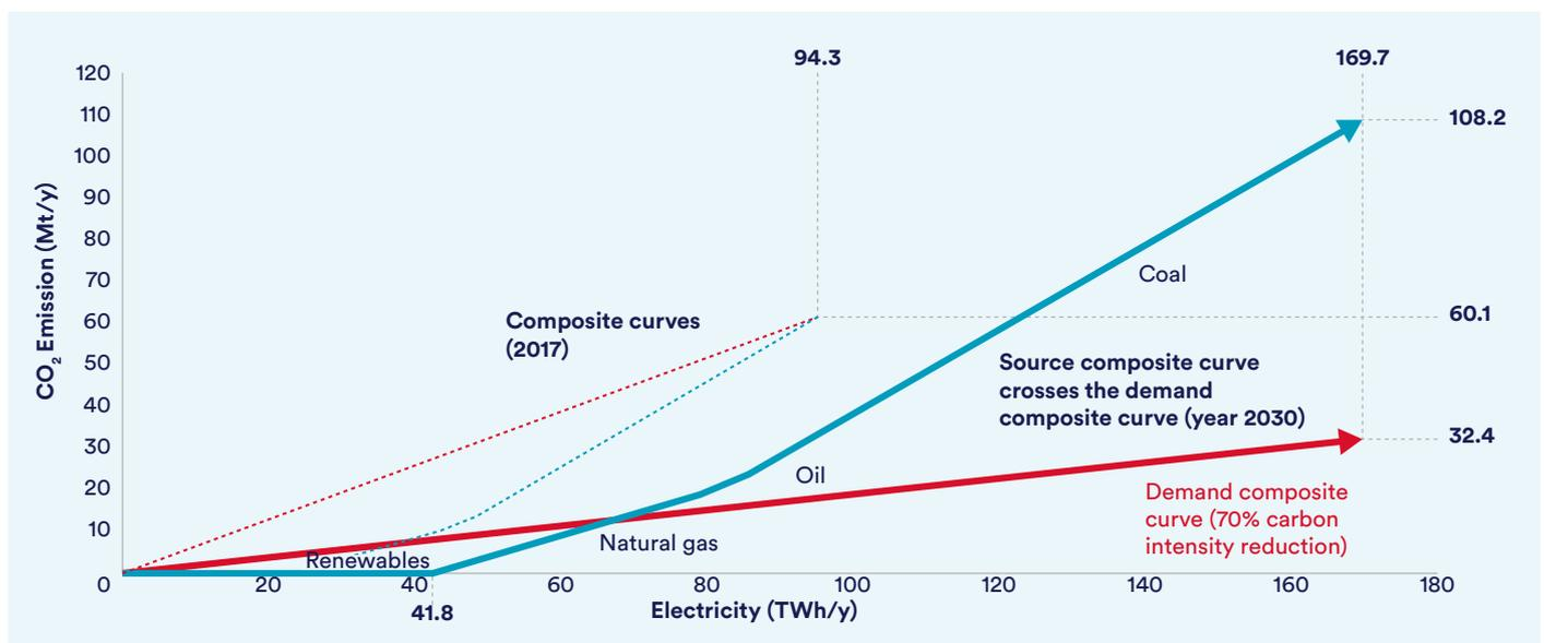
Figure 3. Carbon-energy diagram for year 2030, with 117.5 TWh from zero-carbon power plants, leaving just 8.5 TWh from coal-fired power plants
