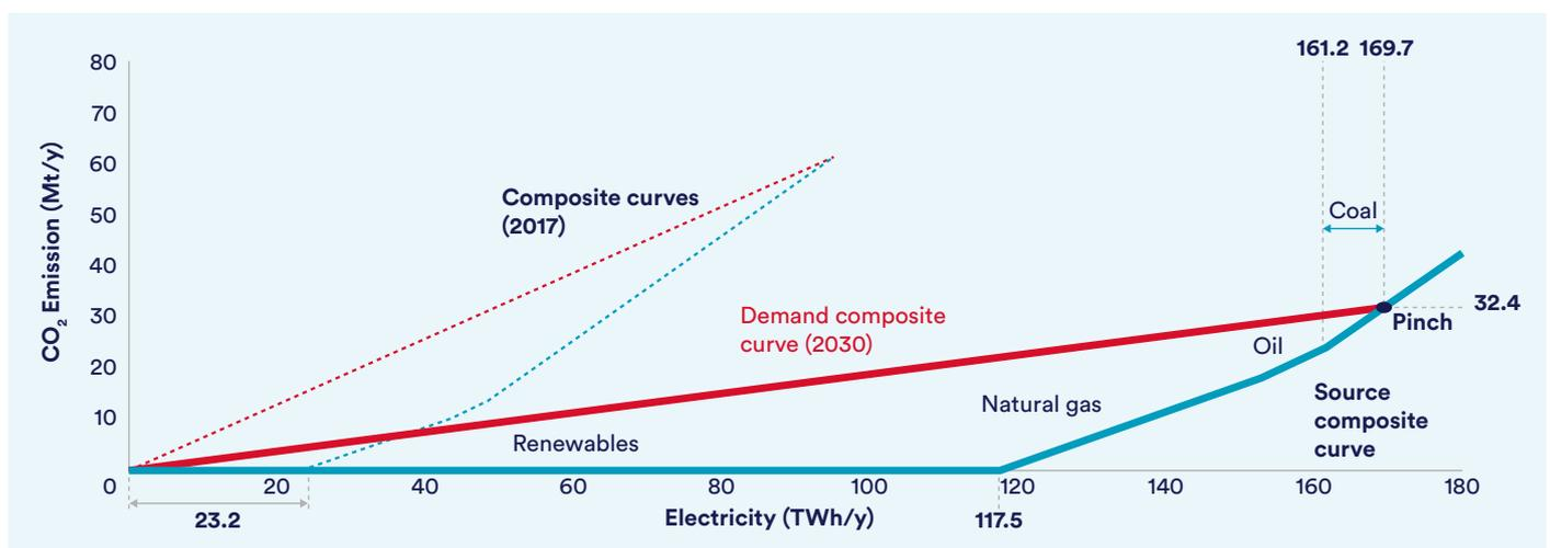
Figure 4. Carbon-energy diagram with NET implementation, with 92 TWh from zero-carbon power plants, with 14 TWh from coal-fired power plants
