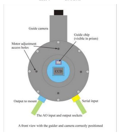
The SXV-AO can execute an image position correction in a few milliseconds, but the effective correction rate is limited by the brightness of the guide star and the download speed of the guide camera image. For best results with a poor telescope mount, you need to choose as bright a star as possible and use a small guide window. Binning the guide camera image will also help.
