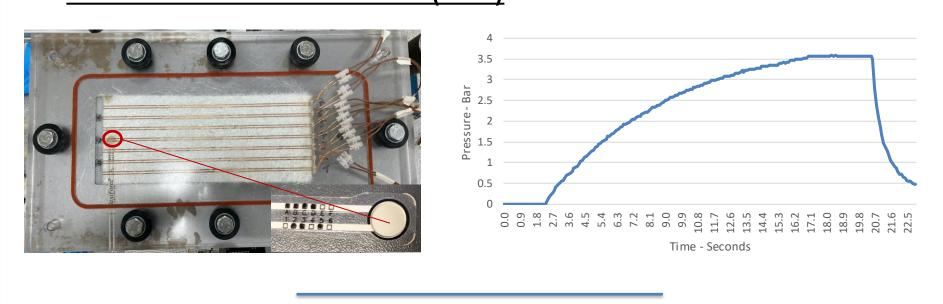
Multi-point FSR sensor / Pressure mapping sensor
