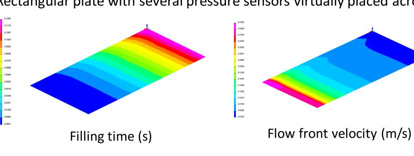
Rectangular plate with a low-permeability channel creating a preferential flow path for the resin (a phenomenon called race-tracking), several pressure sensors virtually placed in the channel and in the middle of the preform
