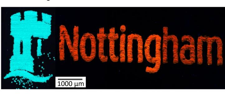
Printed green CsPbBr<sub>3</sub>/graphene composite on Kapton and glass:
