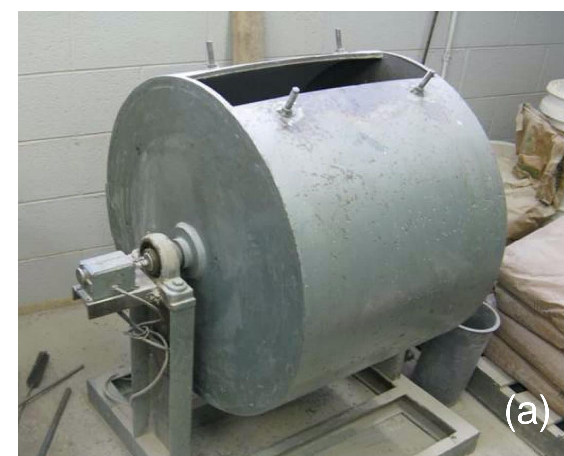
Figure 4. Cantabro test: (a) Los Angeles drum; (b) illustration of operation inside the drum [6]
