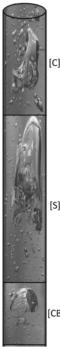
Stacked High-Speed Camera (HSC) images of cap bubble, slug and churn flows for a gas-oil mixture in a transparent vertical pipe
