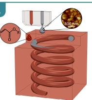
The Dragonfly LDM printer by Nano Dimension is the best-in-industry for IJP electronics. It uses a UV-curable polyacrylate to support Ag structures made from an infra-red-sintered NP ink, and is the basis for this project.
