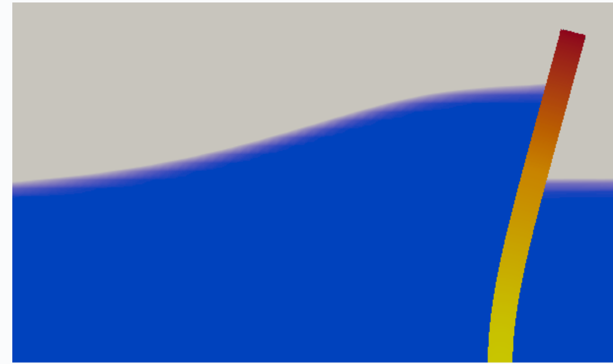
Fig. 2. Numerical simulation of a solitary wave impacting a flexible plate.
