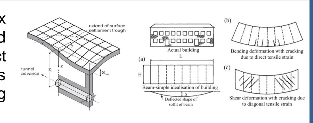
**Aim:** This project aims to investigate the tunnel-soil-structure interaction as well as tunnelling-induced building deflection pattern and damage category by adopting the coupled centrifuge-numerical modelling method (CCNM), a novel hybrid testing approach developed in Nottingham.
