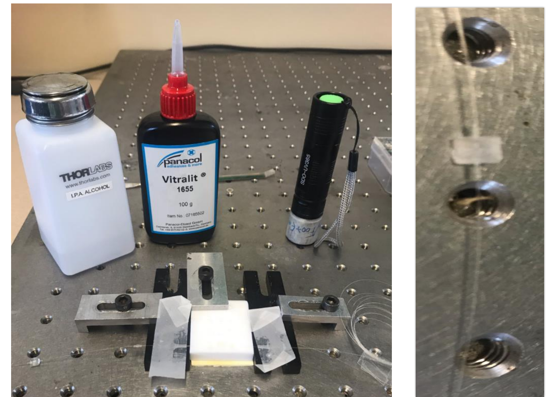
Figure 3: Polymer SYLGARD is poured into a white 4mmx4mm mould (left) with the fibre (with the FBG inscribed) placed in the centre. After the polymer has cured the sensor (right) is ready to be calibrated.
