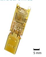
A USB stick allowing detailed component analysis and defect detection
