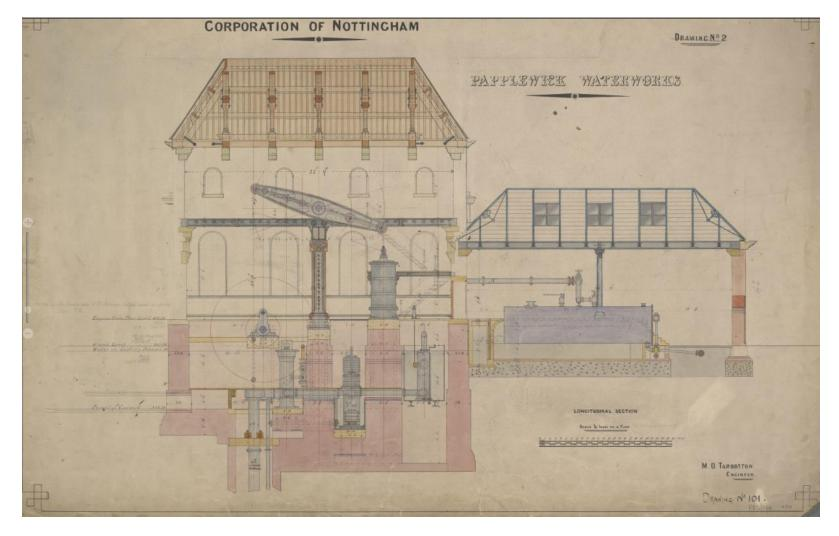
Longitudinal section of Papplewick Pumping Station engine house and boiler house showing beam engines, drawn by M.O. Tarbotton, Engineer, for Nottingham Corporation, c.1883
