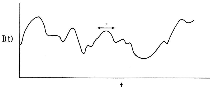
Fig. 1. Fluctuation in scattered intensity,  $I(t)$  with time,  $t$ . The variable  $\tau$  is defined as the "delay time." At short delay times, there is good correlation in the scattered intensity; at long delay times, poor correlation.
