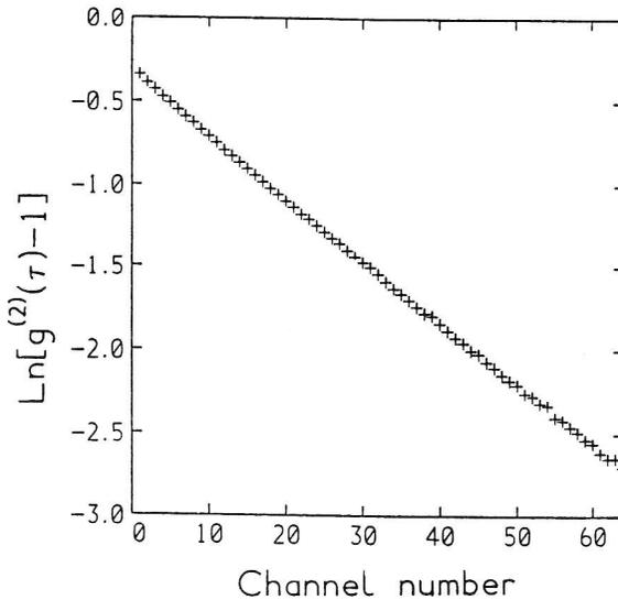
Fig. 2. Plot of  $\text{Ln}[g^{(2)}(\tau) - 1]$  vs “channel number” for the protein assembly dynein.  $\tau$  is the delay time;  $g^2(\tau)$  is the normalized autocorrelation function; “Channel number” = delay time/sample time.
