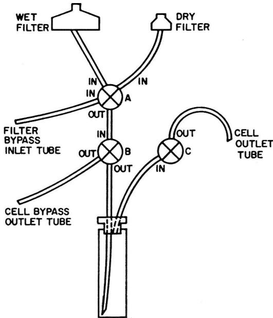
Fig. 4. Schematic cell filling apparatus for minimizing supramolecular contamination (reprinted with permission from ref. 17).
