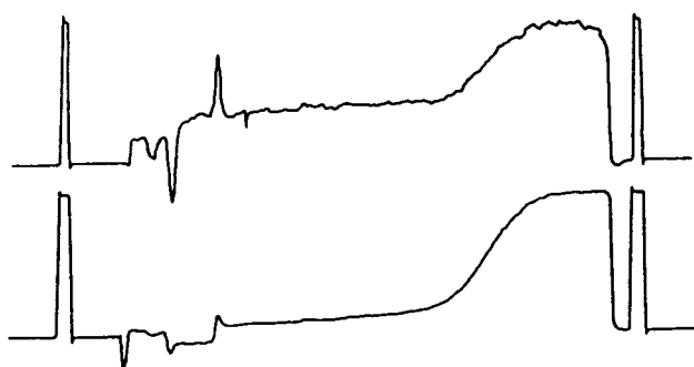
Fig. 4. Co-sedimentation diagram (at 44 000 rev/min) for an enzyme (methyl-malonyl mutase), scanned at 295 nm and (top) its B12 co-factor, scanned 2 min later at 608 nm. The centre of the sedimenting boundary is virtually the same for both, with no residual absorbance, confirming complete binding of the co-factor to the enzyme.
