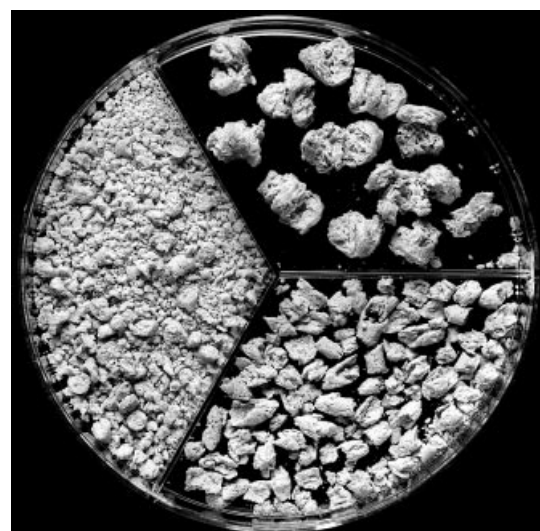
Figure 5. Extrusion products from wild-type and mutant pea flours. Pea flours of (clockwise from top) wild-type and mutants r and rug3 sim32 were extruded using a Clextral BC21 twin-screw extruder (screw speed 200rpm). Moisture contents in the extruder (assuming 10% moisture in the original flours) were 18.8, 19.6 and 24.1% for wild-type, r and rug3 sim32 respectively. The maximum temperatures recorded at the die (3mm) were 86, 87 and 86°C respectively. A cutter (4500rpm) was fitted to generate small, intact pieces suitable for feeding to poultry.
