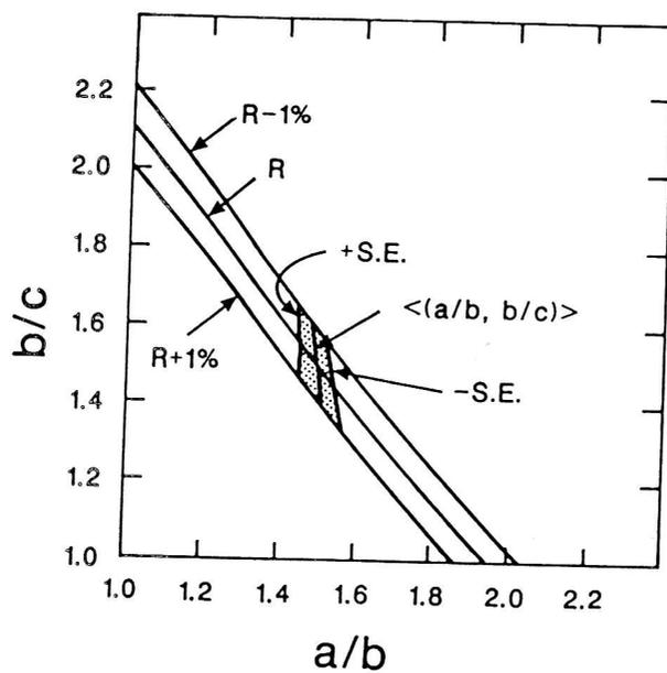
**Figure 10** Constrained non-linear least squares fit of electric birefringence decay data. The plots are of constant  $R$  in the  $(a/b, b/c)$  plane corresponding to an  $(a/b, b/c)$  of  $(1.5, 1.5)$ . Shaded area corresponds to allowed band of axial ratios obtained by constraining the estimates for the  $\delta_+$  and  $\delta_-$  functions to lie on the  $R$  curves. Simulated data, true  $(a/b, b/c) = (1.5, 1.5)$ ; 0.1 deg. random standard error on the birefringence decay data.
