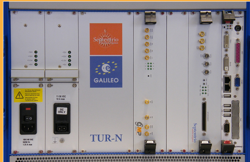
Figure 1 • Septentrio Test User Receiver (TUR-N) developed for the Galileo Test User Segment
