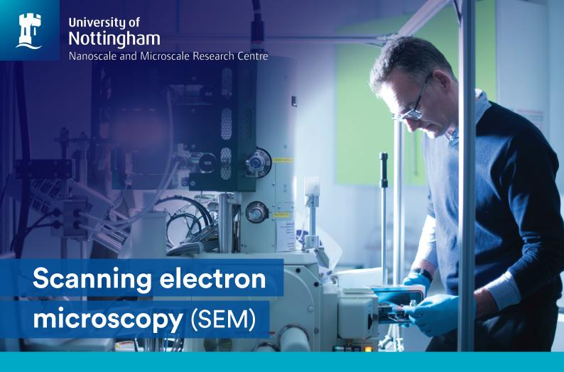
**Scanning electron microscopy** uses a beam of electrons to characterise the topography and structure of a sample. High depth of field images with a 3D perspective and lateral resolutions down to 1-nm can be supplemented with simultaneous chemical and mechanical data.
