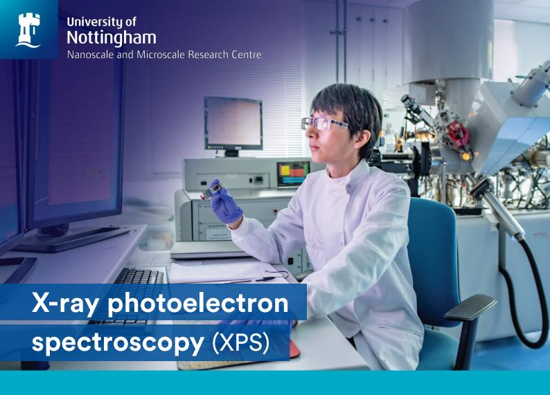
X-ray photoelectron spectroscopy provides a quantitative measurement of surface (5-10 nm) elemental composition and chemical state using X-ray stimulated photoelectron emission.
