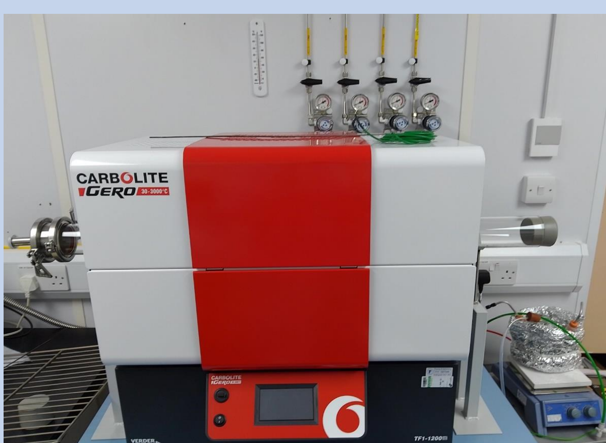
Thermal treatment: Carbolite Gero furnace, rapid thermal annealer, Purged hotplates
