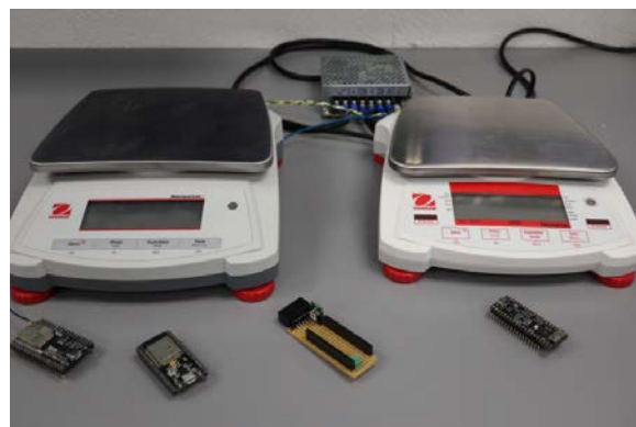
MakerSpace electronics: This project uses "internet-of-things" technology to modify laboratory balances for automated weight monitoring in long-term experiments. These low-cost devices are also being used to develop wireless environmental sensor networks
