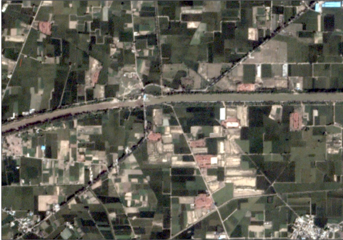
Figure 1: An example of brick kilns located in Punjab, India – note the distinctive red colour which contrasts with the fields surrounding the structures. 4-band PlanetScope Scene projected in true colour with 3m resolution. Imagery captured September 2018. Copyright 2018 Planet Labs. 82
