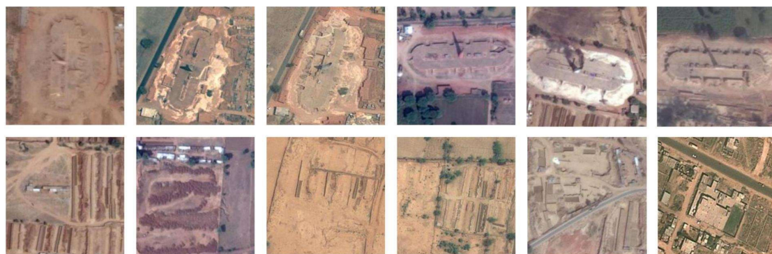
Figure 4. Examples of training samples used in the convolution neural networks (CNN) analysis. The top row of images shows examples with brick kilns while the bottom row shows non-kilns samples. Image data shown from Google Earth provided by Digital Globe.
