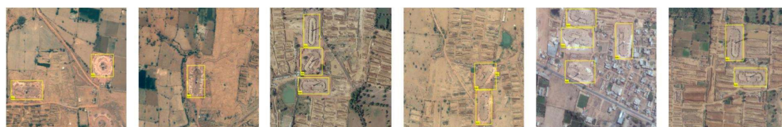
Figure 3. Examples of training samples used in the Faster-RCNN analysis. The yellow rectangles identify kilns in the images. Image data shown from Google Earth provided by Digital Globe.
