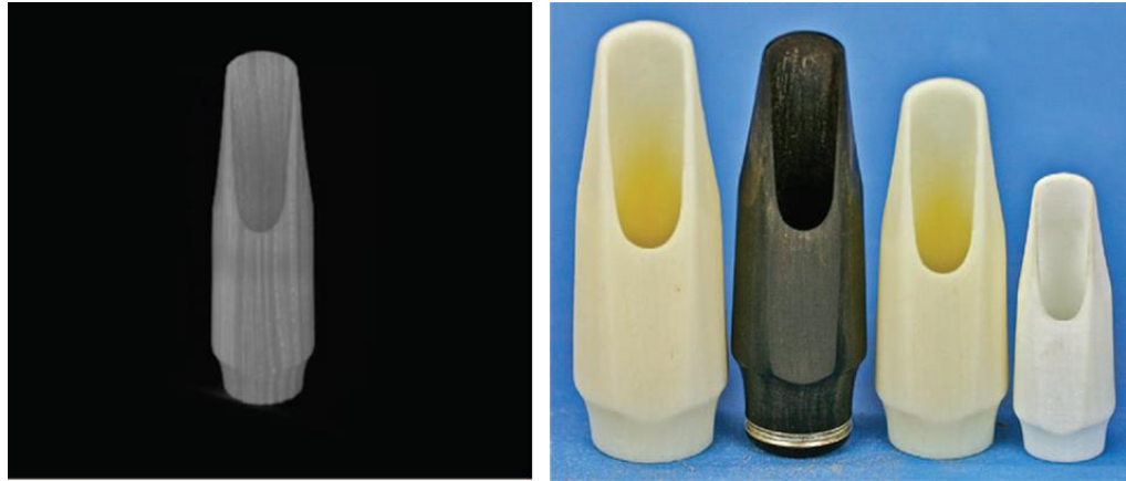
Figure 2.4. Left: XCT data of a saxophone mouthpiece, right: AM reproduced saxophone mouthpieces with original wooden mouthpiece (second from left). All the AM mouthpieces were produced by scaling of the original scan data and the rightmost mouthpiece was stated to be sufficiently dense as to operate successfully. Figure published in [1].
