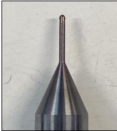
Figure 19: Ballnose tool used to produce the callotes.
