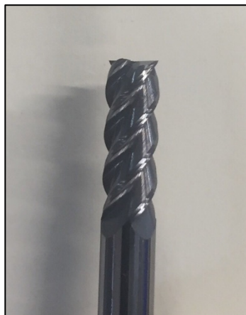
Figure 18: carbide end mill tool used to flatten the top surface of the artefact.
