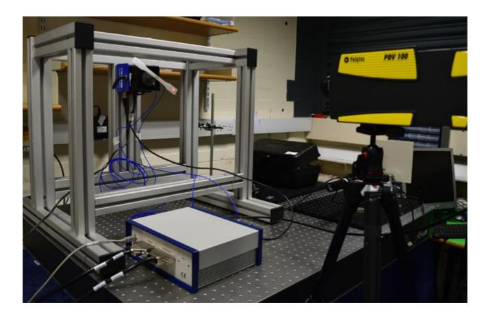
Vibration generated at the centre of an additively manufactured test sample by the piezo accelerator while vibration of the sample tip is being measured by the laser vibrometer.
