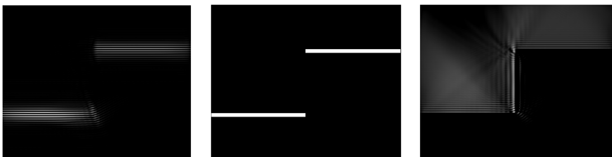
Figure 3 Left: measured CSI interferogram. Centre: finite element model from CSI interferogram. Right: second-order CSI interferogram, clearly showing the vertical sidewall (results from work at Loughborough University)
