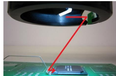
CCD-based in-line metrology solution
