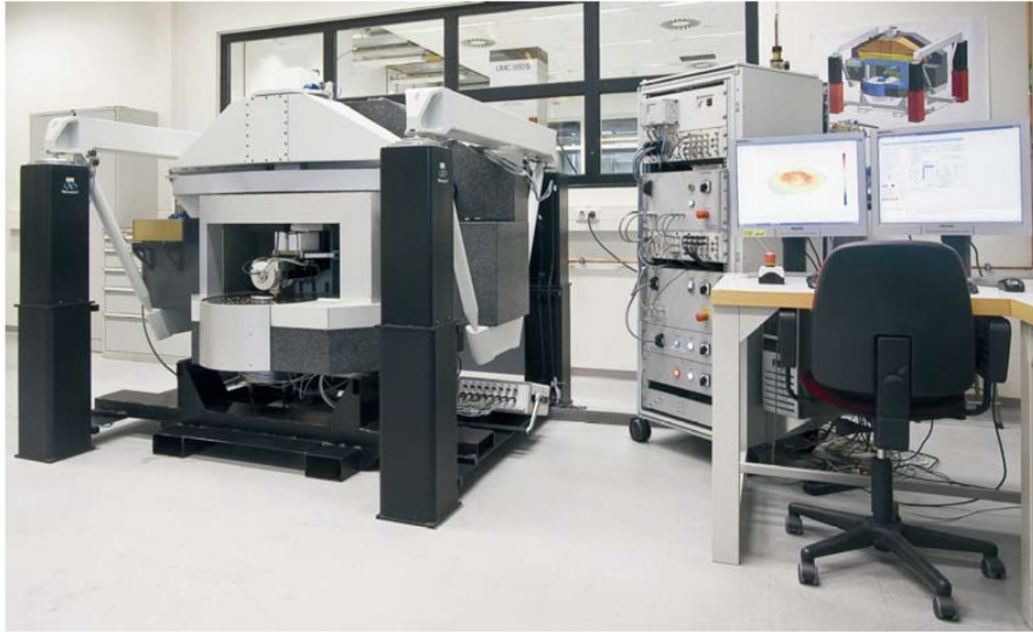
Figure 2.25 Non-contact freeform optics measurement machine prototype (Henselmans, 2009)
