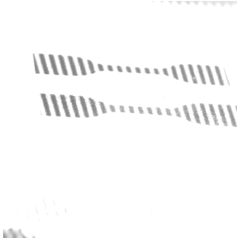
(b) First phase shift high frequency fringe image from layer 22. The image is overexposed, but the layer before was correctly exposed.
