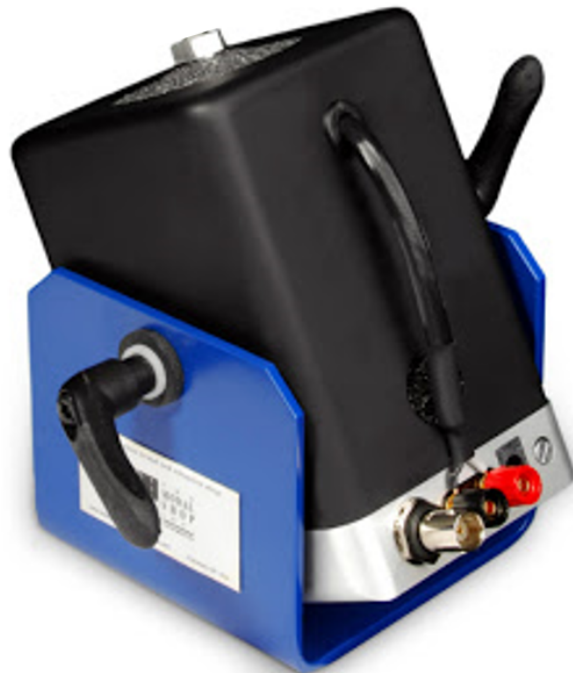
Figure. 3.3 The Modal Shop smart shaker K2007E01 [1] that was used to excite the different structures in each vibration experiment
