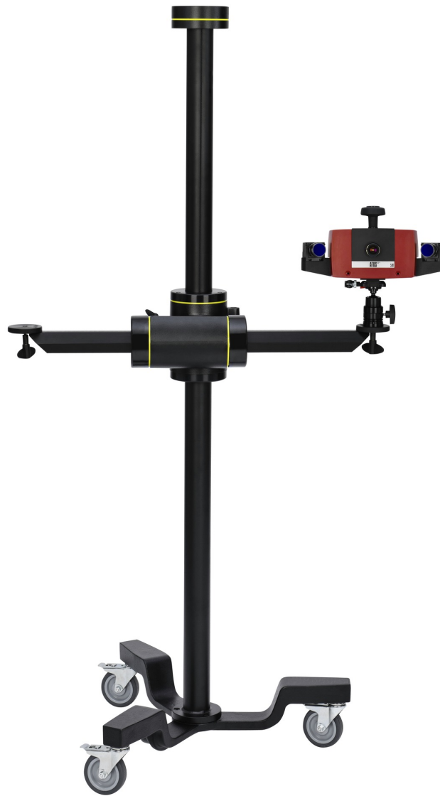
Figure. 2.14 Example of a commercially available fringe projection system mounted on a tripod.
