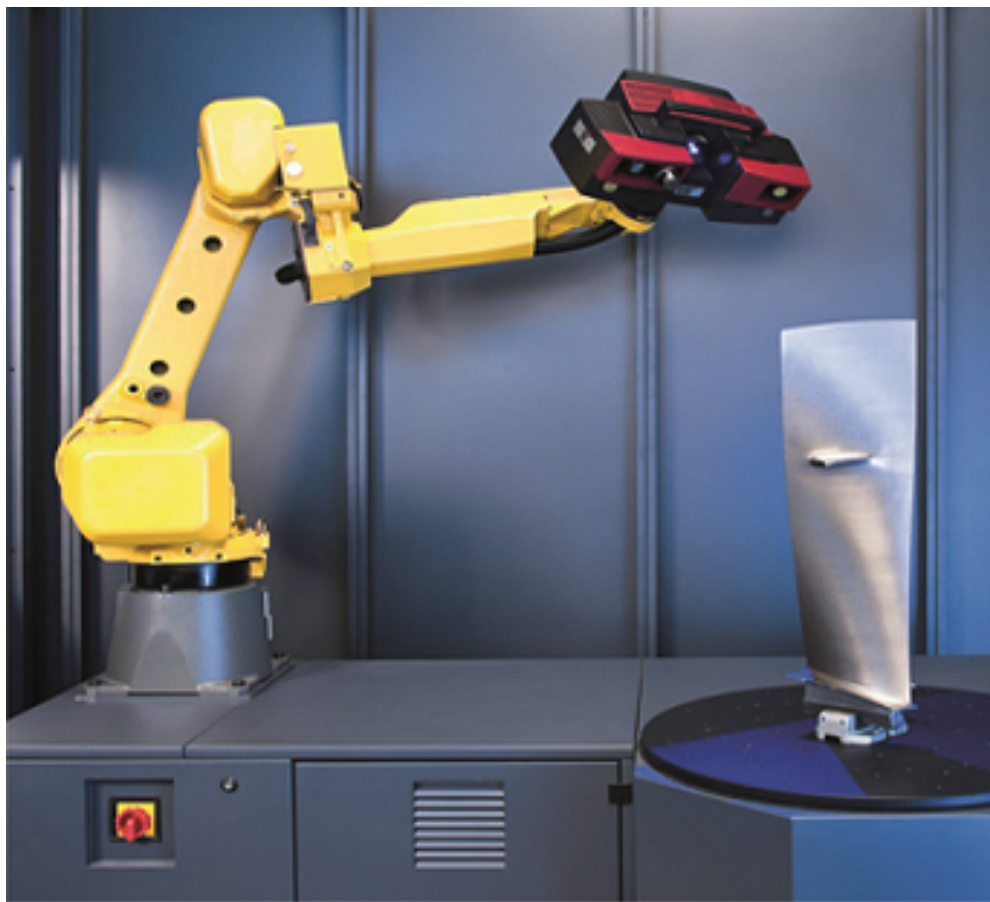
Figure. 2.13 Example of a commercially available fringe projection system mounted on a robot arm.
